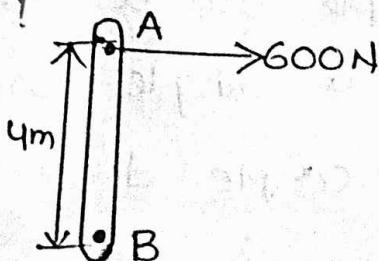
COUPLE : Two non-collinear parallel forces of equal magnitude and in opposite direction form a couple. Couple produce rotational effect.
