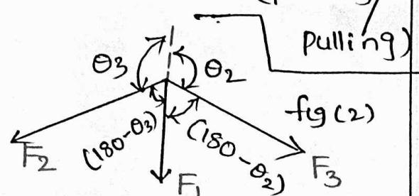
From the above fig (1)  $F_2$  &  $F_3$  forces are pulling forces but ' $F_1$ ' is pushing force. By principle of transmissibility, one can transmit  $F_1$  on other side of point of concurrency to make three forces same nature.
