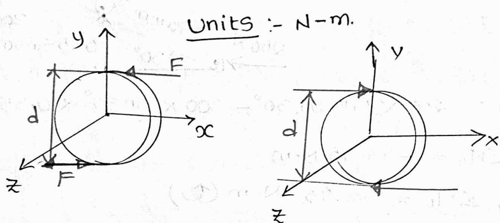
Moment of a couple is the product of common magnitude of two forces 'F' and of the perpendicular distance 'd' between the lines of action.
